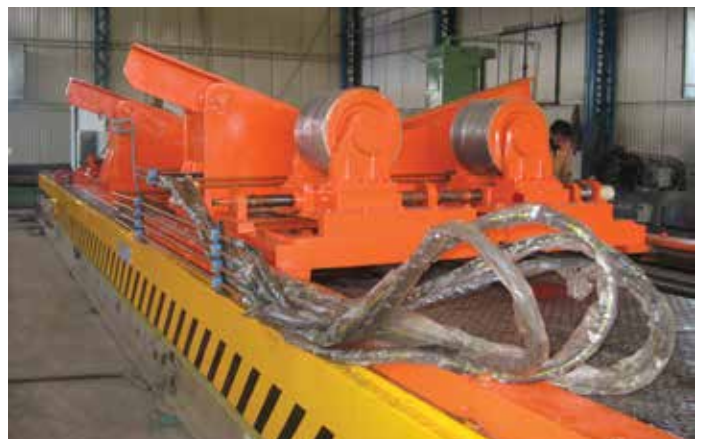
Pipe Carriage for UT & X-ray Test
